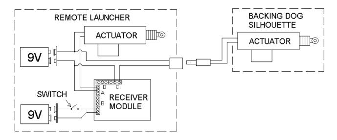
The receiver could be mounted on one device, like a launcher, then connected to other devices using lengths of wire and jacks. Wired like this, the C channel would be used to raise the backing dog silhouette, and the A channel would release the bird.
